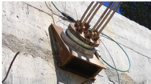
Borehole extensometer, anchor load cell, clinometer
