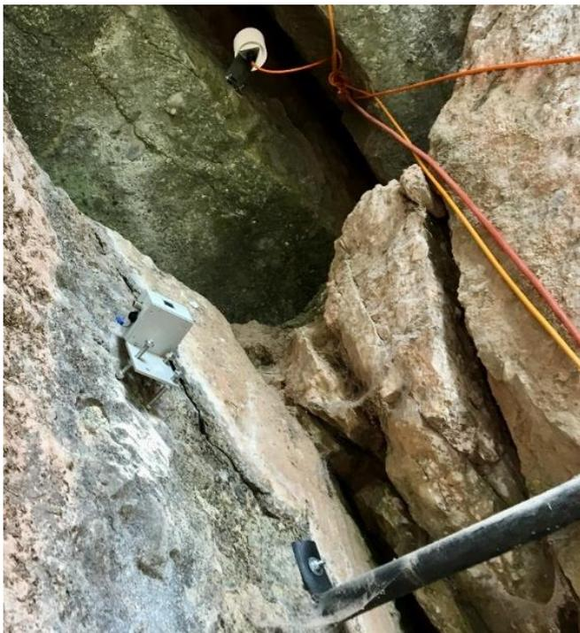
Laser distance measurement sensor
